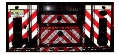
The back of the bus should include red and white striping, with the above picture showing the correct direction of the striping, A shaped, not V shaped.
